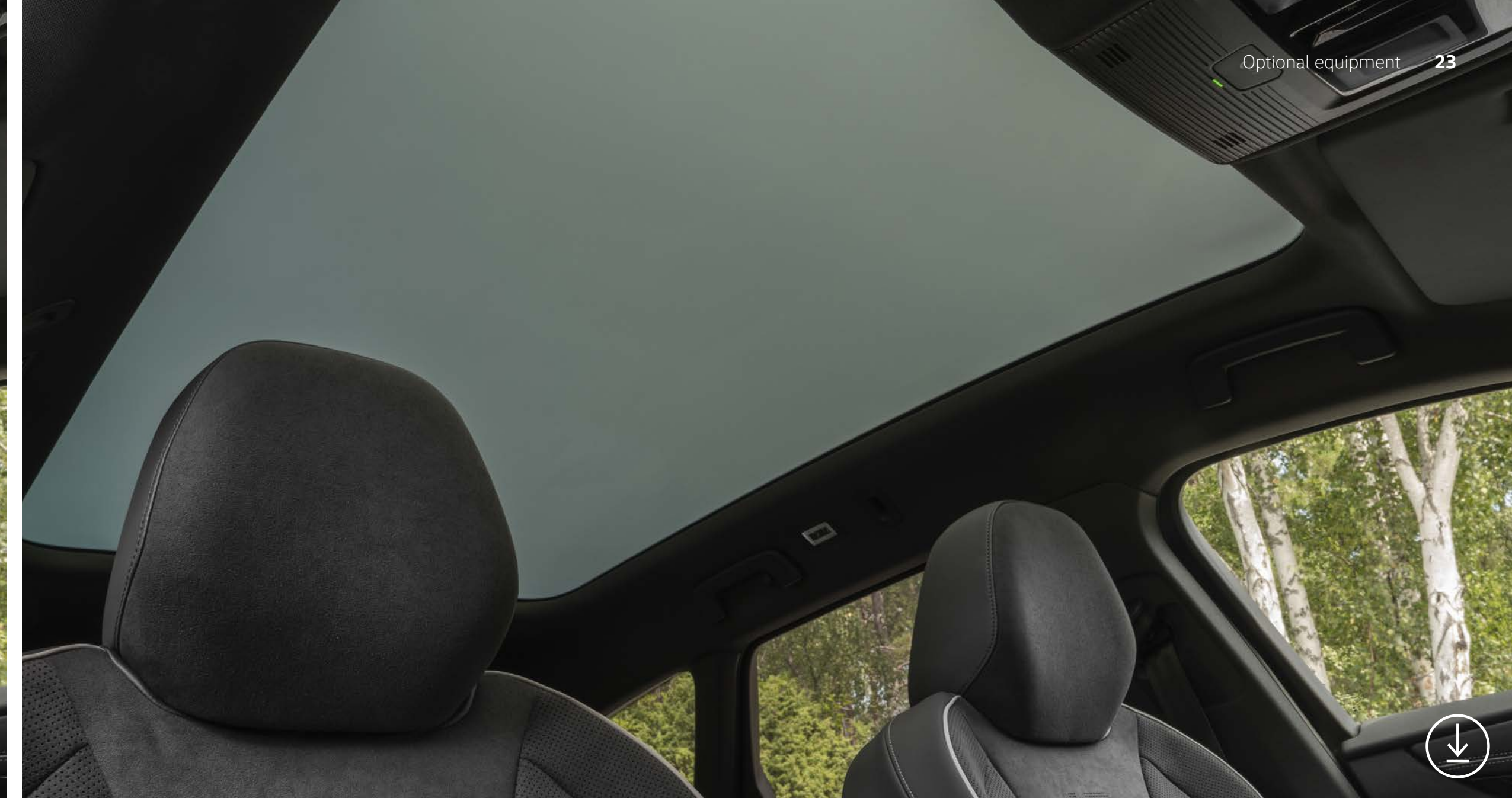
Smart Glass 12 in opaque setting.
