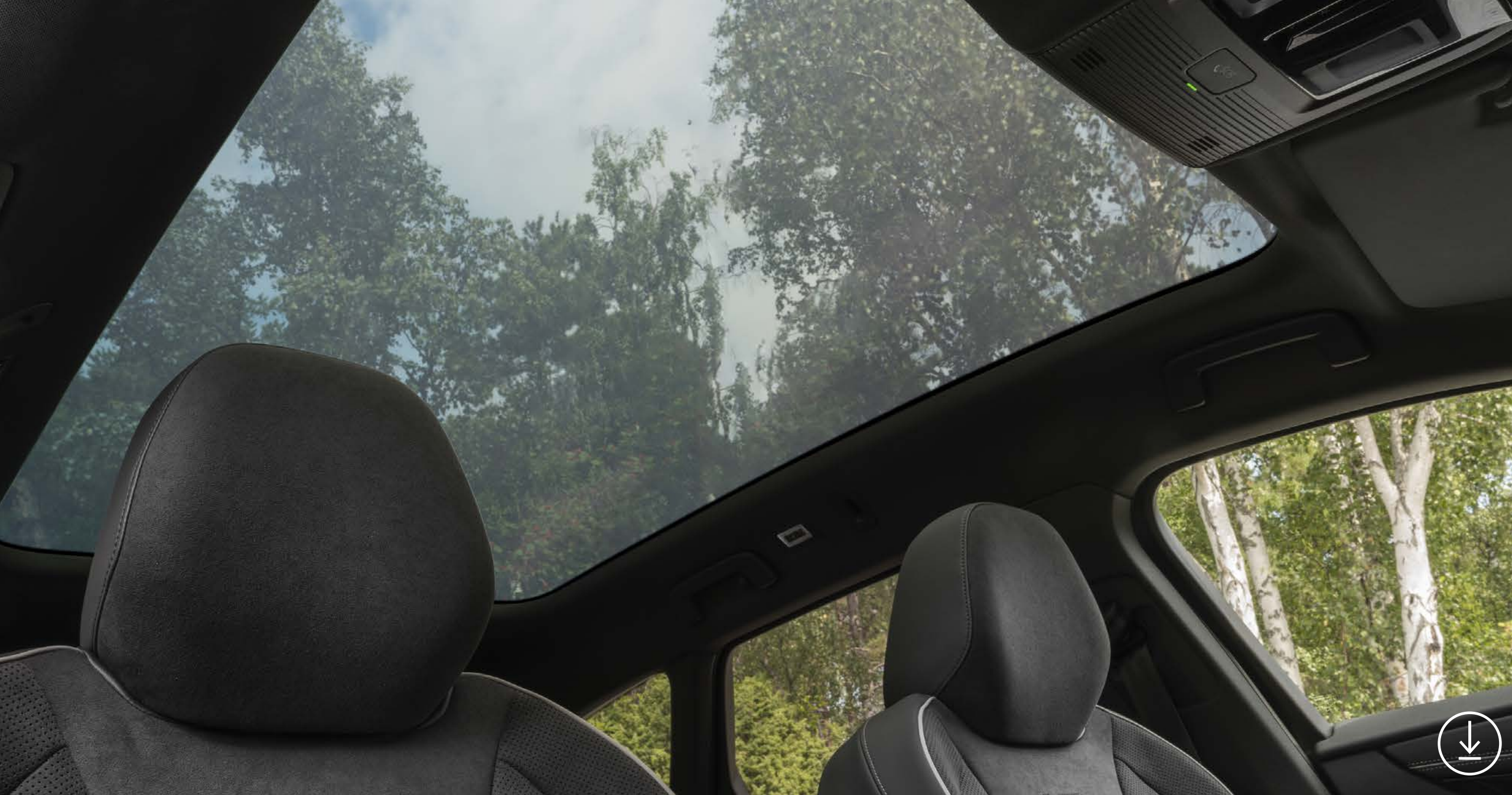
Smart Glass 12 in transparent setting.
